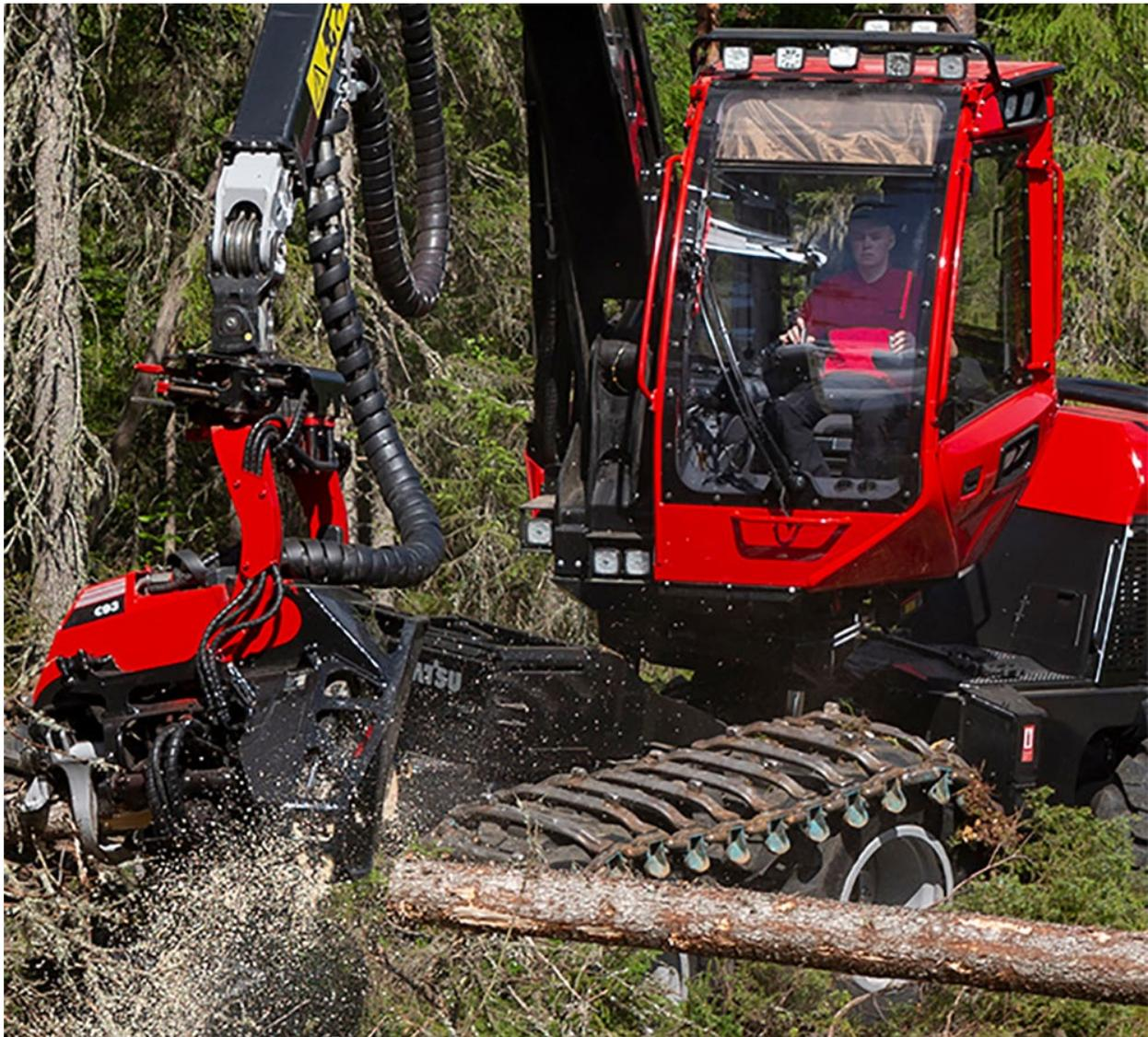
The modern, comfortable 901XC cab features excellent upward/downward front line-of-sight visibility, 4-way cab/crane leveling and  $\pm 180^\circ$  cab/crane rotation.
