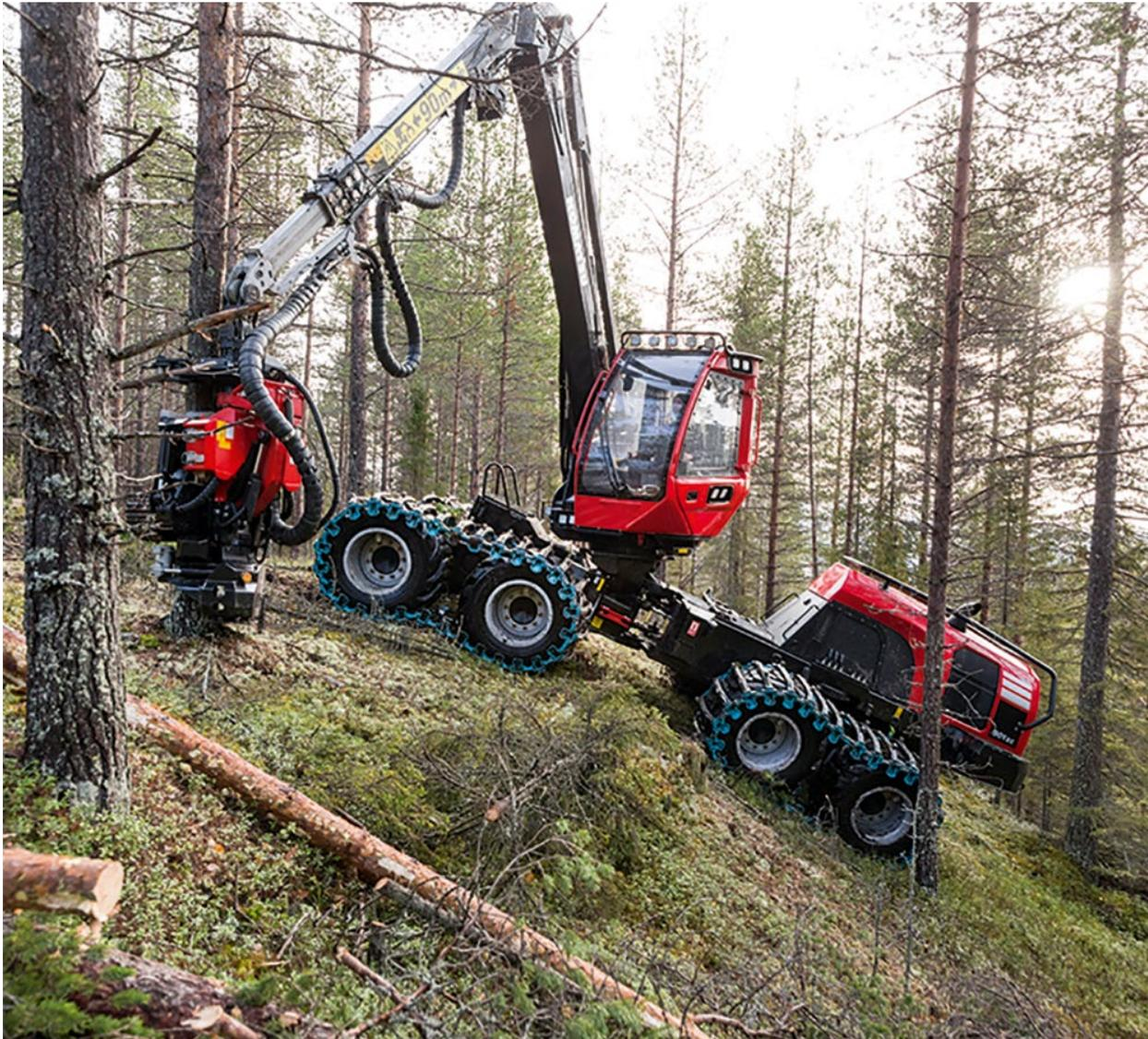
**The new Komatsu 901XC is a Thinning Powerhouse featuring a unique double Komatsu Comfort Bogie 8WD system designed to tackle steep, rough and soft terrain.**
